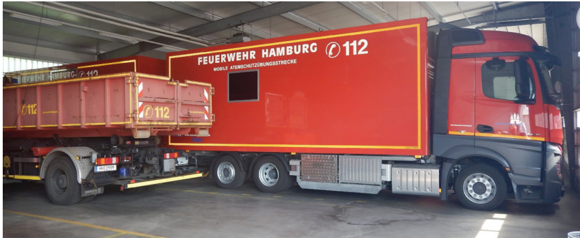
Picture 22: Firefighter practice track in a vehicle combination at the Firefighting Academy of Hamburg, Germany
