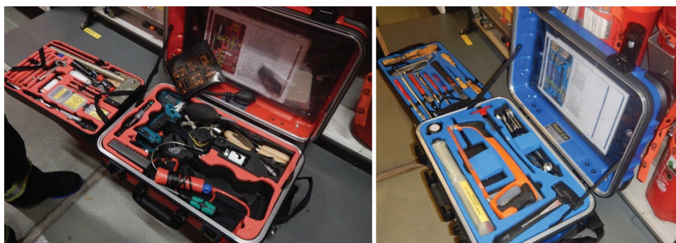
Picture 36–37: Compact, well-equipped tool cases with space-saving in a fire engine in Berlin, Germany
