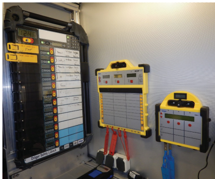
Picture 15: Different types of Draeger respiratory telemetric systems in Blyth, United Kingdom
