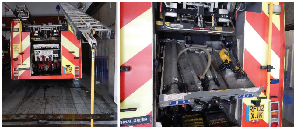
Picture 12–13: Handles and lifted/tilted shelves for easier access of the fire equipment in London, United Kingdom
