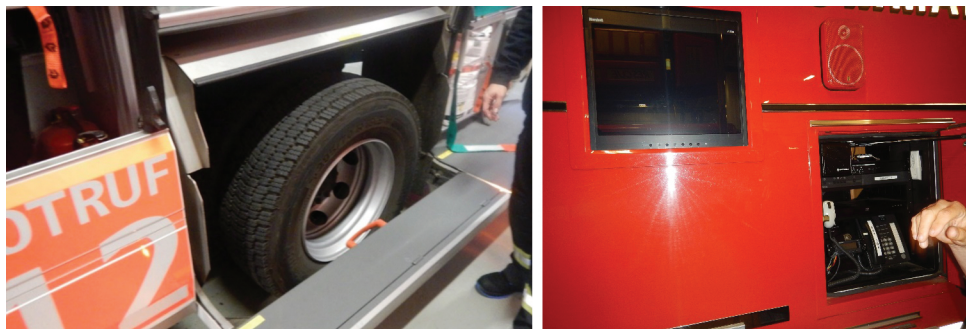
Picture 34–35: Using all spaces in a fire truck to install mobile steps in Berlin, Germany and outside control, display possibilities in a fire incident commander vehicle in Washington, D.C., United States
