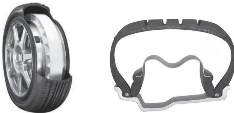
Picture 8. Run-flat tire with support ring. [29]
