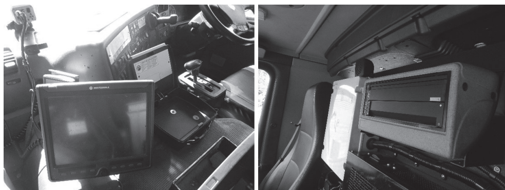
Picture 12. (left) and 13. (right) Mobile Data Terminal and its thermal printer integrated in a fire engine, Liverpool, United Kingdom, 2017. [Author's own photos.]
