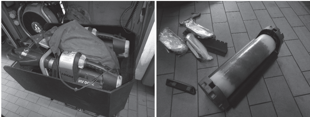
Picture 8. (left) and 9. (right) Electronic spreader-cutters and highly durable, colour-coded protection Packexe film in a fire engine in Liverpool, United Kingdom, 2017. [Author's own photos.]
