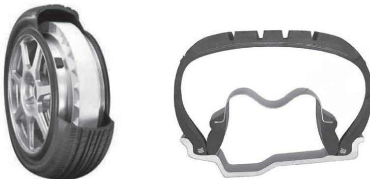
Picture 8. Run-flat tire with support ring. [29]
