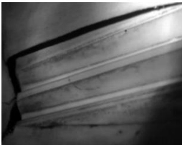
Picture 12. Crack on an annular gear detected liquid penetration test [7]
