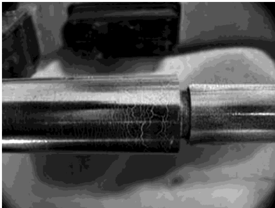
Picture 9. Testing standards to set magnetic particle testing sensitivity [7]
