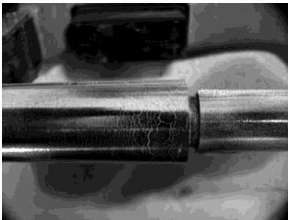
Picture 9. Testing standards to set magnetic particle testing sensitivity [7]
