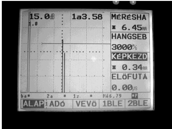
Picture 18. USM-25 ultrasonic testing equipment [7]
