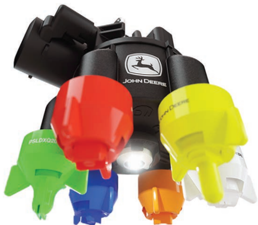
4. ábra: John Deere intelligens fúvókatestje - ExactApply™
