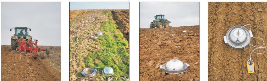
Photos 1–4. Measurement of short-term soil CO 2 emissions (from left to right): tillage implementation (1); inserted circular frames into the soil (2); incubation period (3); measurement of accumulated CO 2 in the chamber (4).
